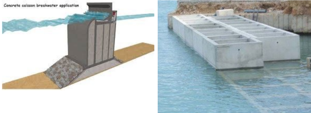
Figure 3.5: Example of typical caisson structure (left) and modular caisson (right)
