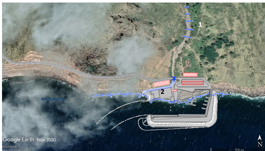
Figure 6.4: Discharge of runoff from weirs: 1. weirs; 2. discharge channel (run-off); 3. Outlet
