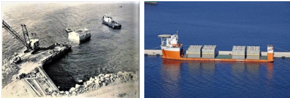
Figure 3.7: Example of caisson transportation by tugs (left; this is a 1970 picture of the construction of the Fort Bay main breakwater), and by semi-submersible vessel (right).
