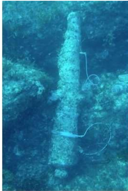
Figure 1: Sample set up of sacrificial zinc anodes to a cannon for in-situ electrolysis (Puoti 2016).
